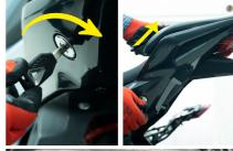
2. Press the lock clips, lift and open the fuse cover as shown.
