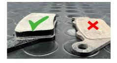
Pulloutthe wornout brake pads and insert the new brake pads. Insert the disc pad lock pin and β clip.
