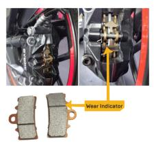
Remove the lock clip using a nose plier and remove the brake pad lock pin using a T30 Torx key and remove the retainer spring and brake pads.
