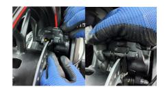
Add fresh DOT 4 brake fluid and pump the rear brake pedal till the brake is loaded.
