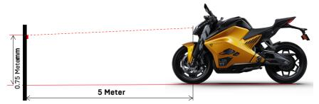
6. Figure below shows an improperly adjusted head light beam, where the beam is below the marked line.
